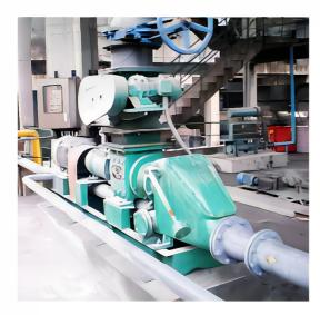
The equipment has the characteristics of compact structure, flexible layout, low wind pressure, low energy consumption, easy operation, reliable operation and so on. It is a product with high performance in low-pressure continuous powder conveying equipment.
