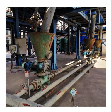
This product is widely used in medium and short-range ash collection and transportation in power ash removal, building materials transportation, construction sites and other industries. It is an excellent product in solid conveying pumps. It is not limited by terrain and elevation difference, fully enclosed, pollution-free, simple structure and small maintenance. The air source is roots blower or compressed air.
